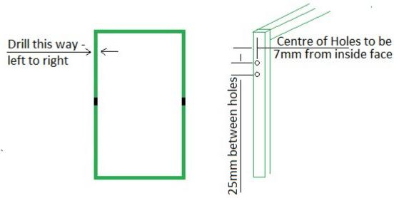
You will need to drill 2 pairs of 5mm holes in the door frame to accept the hinges. Drill left to right, not front to back. The hole centres in each pair should be 25mm apart and 7mm from the inner face of the door frame
