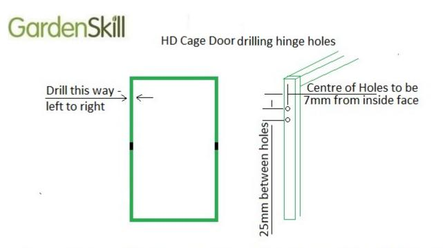
You will need to drill 2 pairs of 5mm holes in the door frame to accept the hinges. Drill left to right, not front to back. The hole centres in each pair should be 25mm apart and 7mm from the inner face of the door frame
